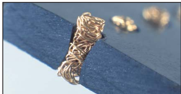
Cross Section of contact in an insulator
